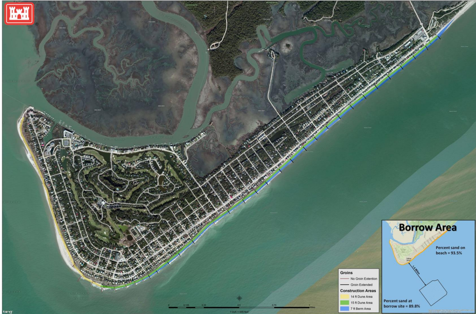
Figure S.2: Primary Features of Recommended Plan
