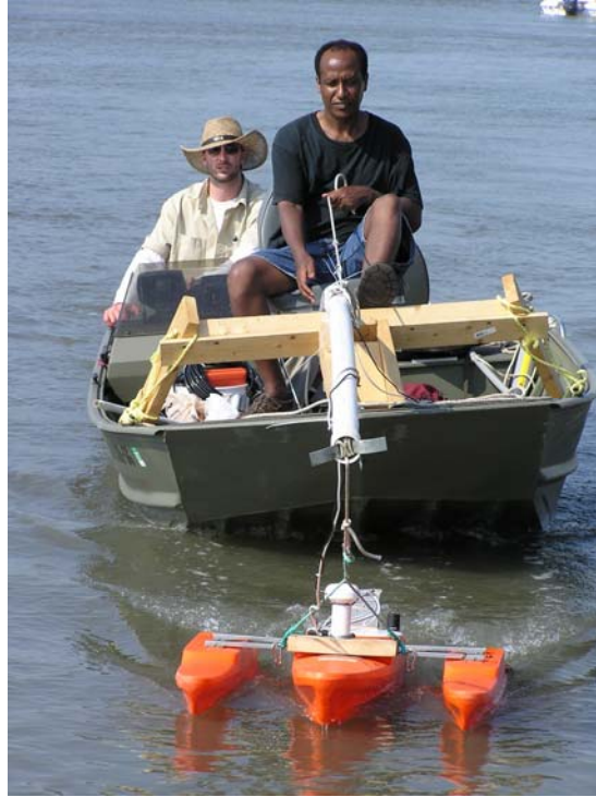
Fig. 19. Forward-push mount and operation for Riverboat trimaran for use with ADCP, equipped with GPS and sonar.
