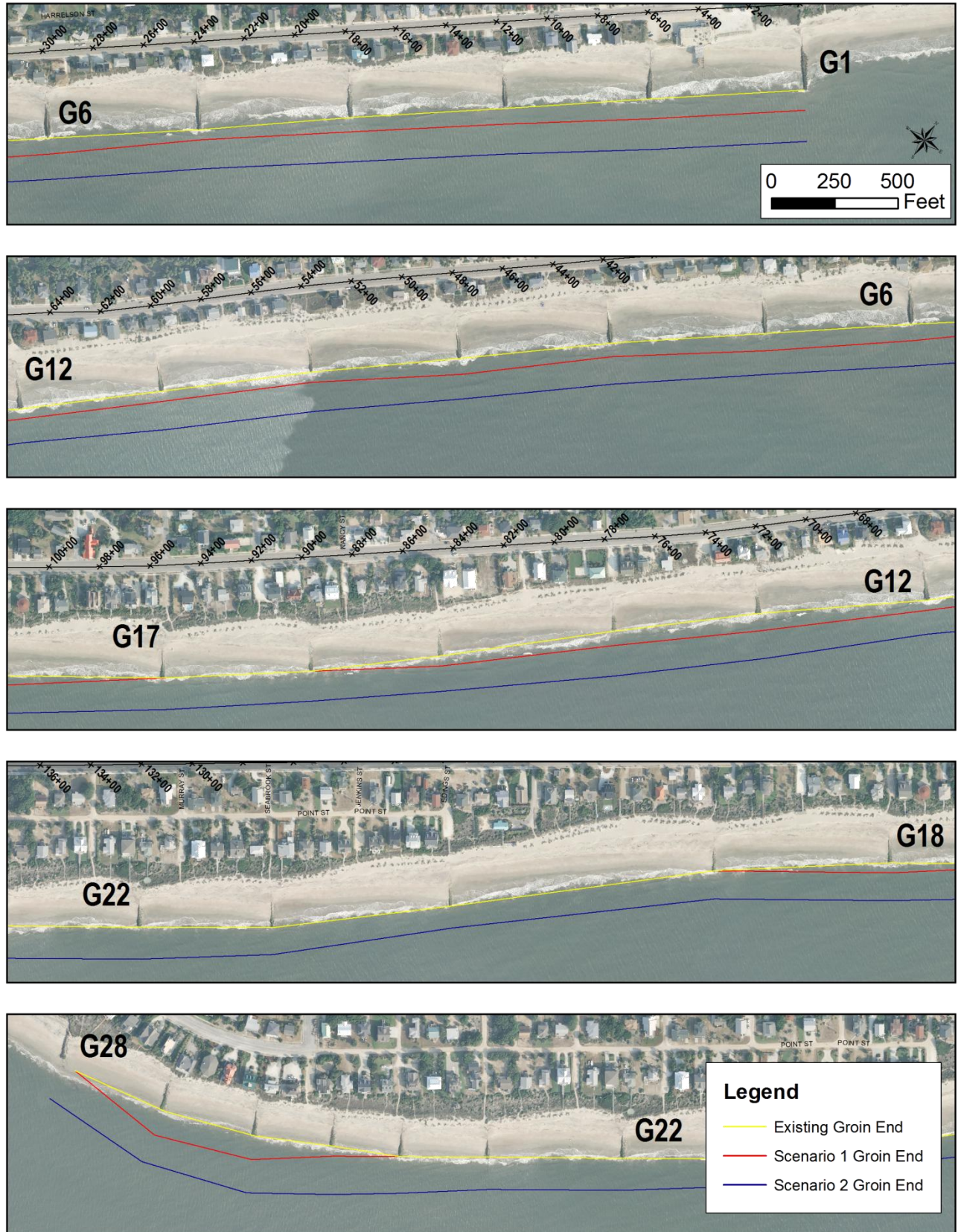
FIGURE 14. Alignment of groin ends under lengthening Scenario 1 and Scenario 2. Where the red line is missing, no groin extension would be completed under Scenario 1.
