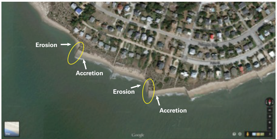
Figure 1. A groin (yellow circle) can trap sand on one side but increase erosion on the other, as seen in this example of Edisto Island (Google Map 2014).
