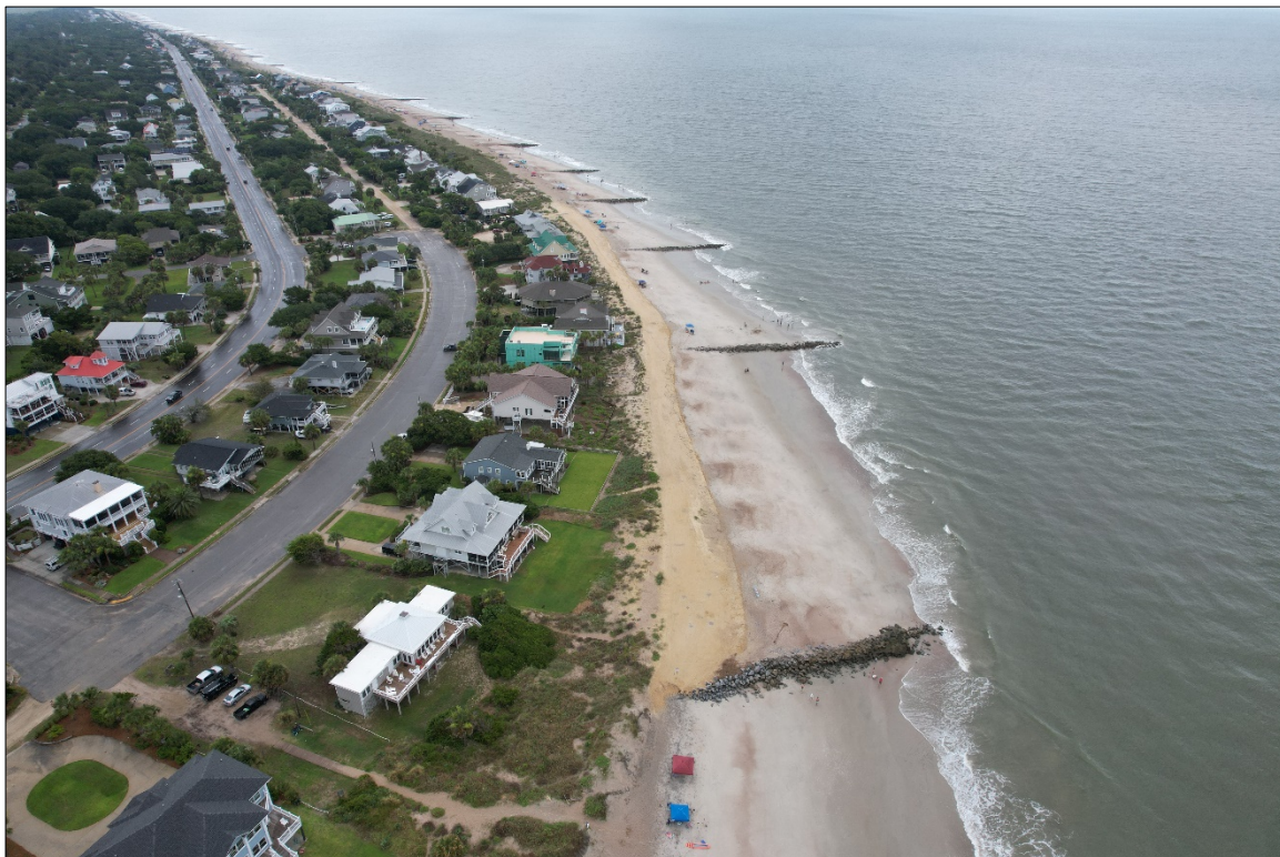
FIGURE 4.13. [UPPER] Aerial view of Reach 4 in January 2019. Groin 28 is in the foreground. [LOWER] The same section of shoreline in August 2021. The beach has equilibrated since the 2017 project with a wider dry sand beach than before construction. The sand used for the dune restoration project is visible. [Photos by D Giles]
