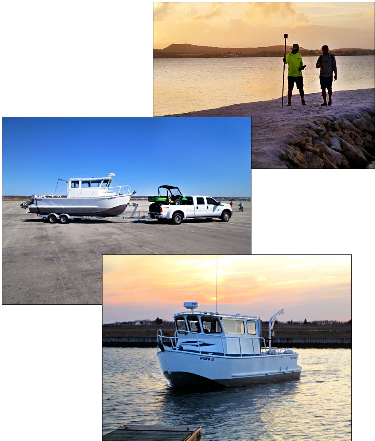
FIGURE 3.2. CSE beach monitoring methods include land-based data collection using Trimble™ RTK-GPS from the backshore to low-tide wading depth and over-water work using RTK-GPS linked to a precision echo sounder aboard CSE's survey boat (R/V Southern Echo ).
