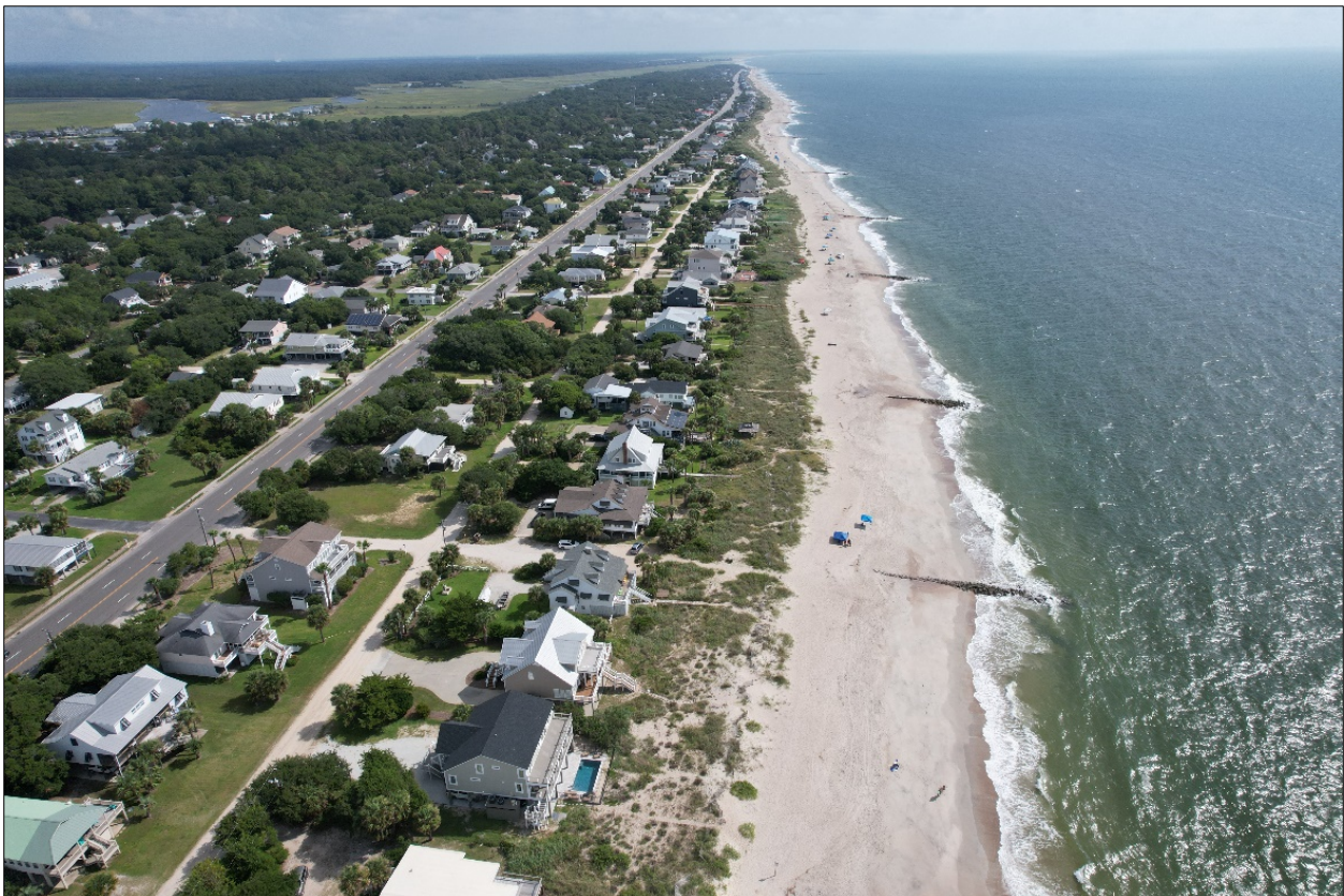
FIGURE 4.10. [UPPER] January 2019 aerial showing Reach 3, which has the greatest setbacks and vegetated buffers of any ocean-facing area along Edisto. Groin 25 is in the foreground. [LOWER] As of August 2021, Reach 3 has remained one of the healthiest portions of Edisto Beach since project completion. Groin 24 is in the foreground [Photos by D Giles]
