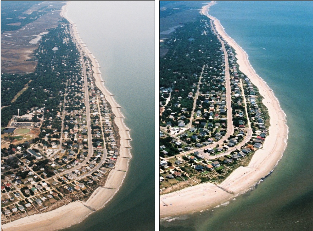
FIGURE 2.5. Aerial photographs showing the state of Edisto Beach before the 2006 renourishment (left, taken by T Kana 10 February 2006) and after project completion (right, T Kana, 9 June 2006). That project resulted in the placement of nearly 900,000 cy of beach-quality material along Edisto Island between the State Park and The Point. Notice the shoreline offset in the background of both images, highlighting the chronic erosion experienced along Edingsville Beach and between Jeremy Inlet and Edisto Beach State Park. This chronic erosion can cause sand deficits along the northern reaches of Edisto Beach itself.
