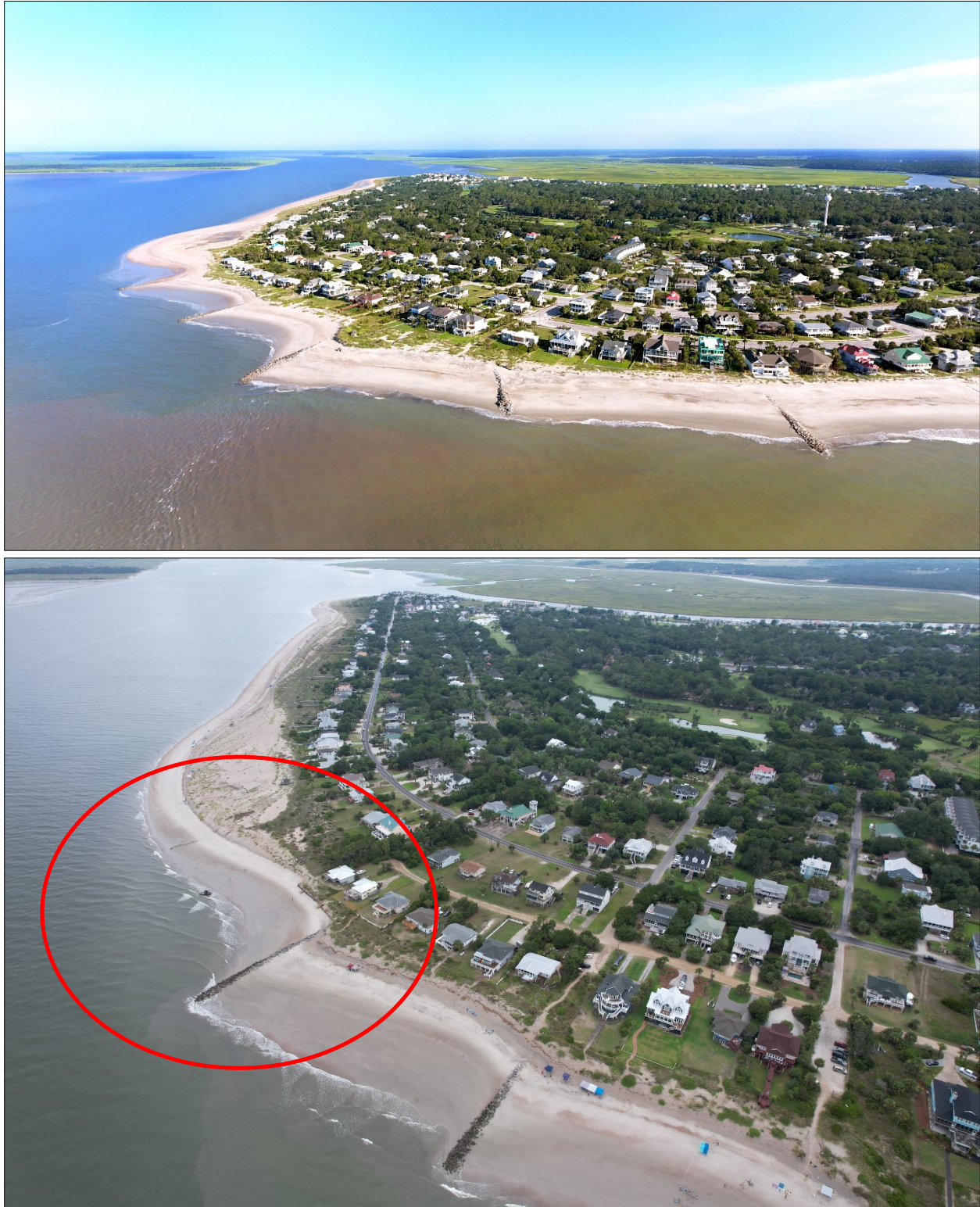
FIGURE 4.16. [UPPER] The downcoast reaches in July 2019. A considerable volume of nourishment sand has made its way around the corner of the shoreline and created a bulge in the beach around the western end of Point St. [LOWER] Reach 4 and downcoast reaches in July 2021. Nourishment sand has continued to move through the groin field to the downcoast reaches, maintaining the prominent bulge along the inlet shoreline, however an erosional arc at groin 31 (highlighted) has resulted in a narrower beach and exposure of a protective wall. [Photos by D Giles]
