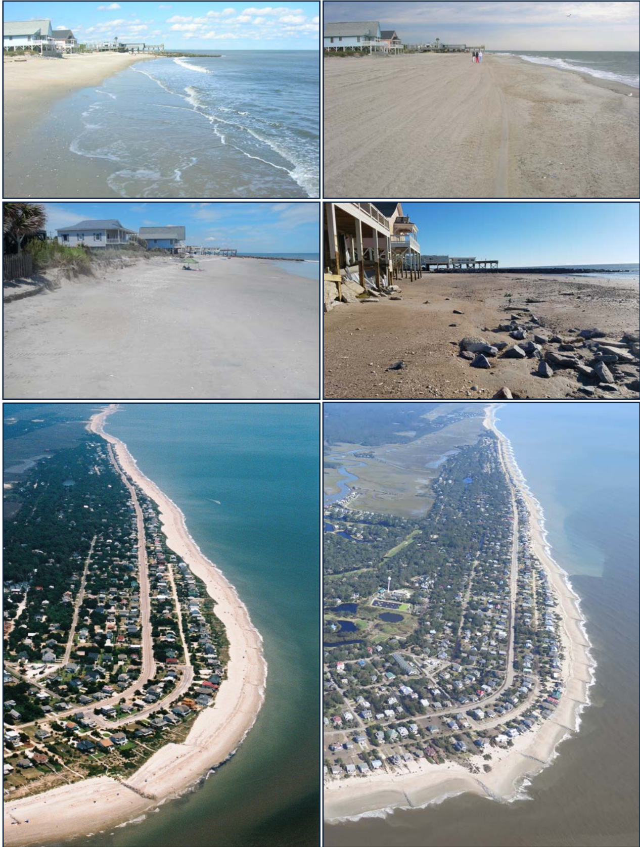
FIGURE 2.9. Image of the beach in the 100 block before (top left) and after (top right) the 2006 project. The middle left and right photos show the same locations in 2016 before and after Hurricane Matthew . The aerial photos show the beach after the 2006 project (lower left) and after Hurricane Matthew in October 2016 (lower right).
